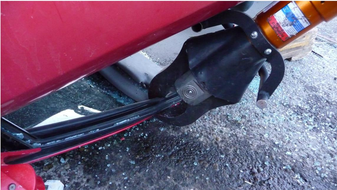
**There should be roughly a 1 inch void from the thickness of the cutter blades that will be enough room to insert the tips of a hydraulic spreader.**
