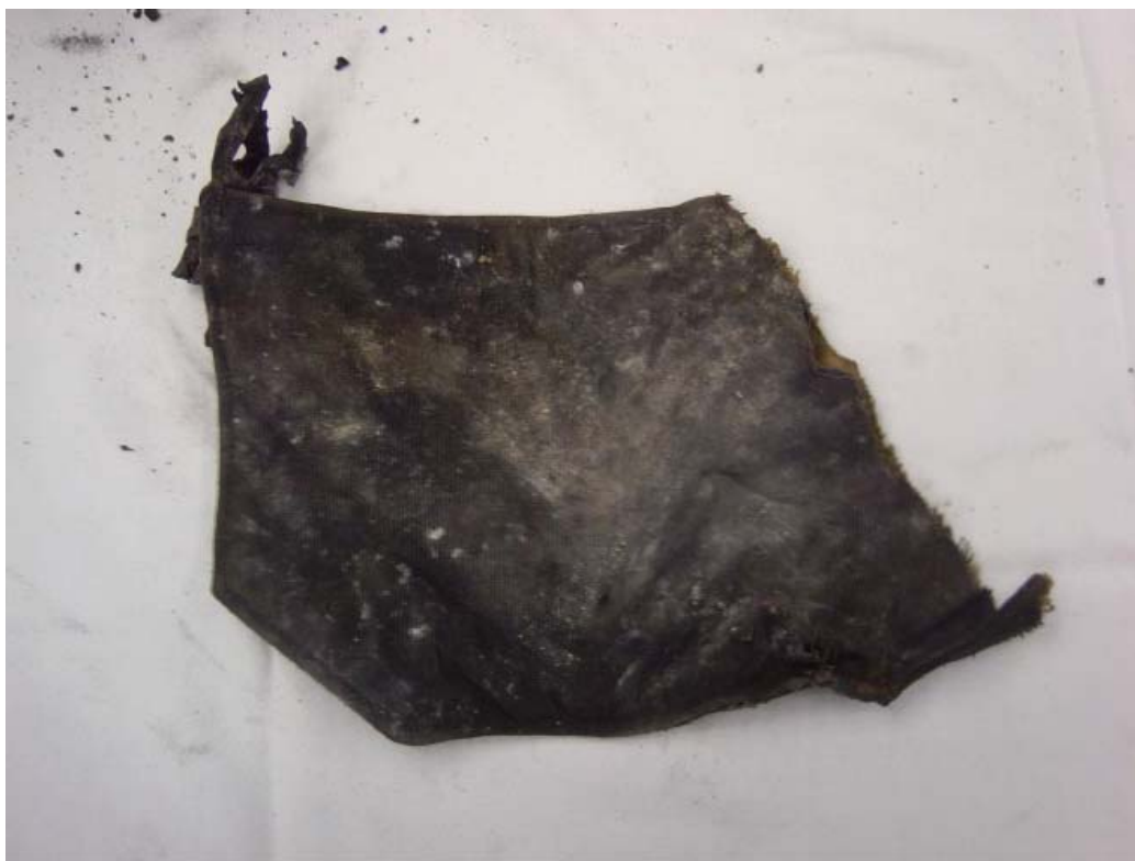
Portion of ear covers carbonized and burned away so Nomex exceeded 750 F.
