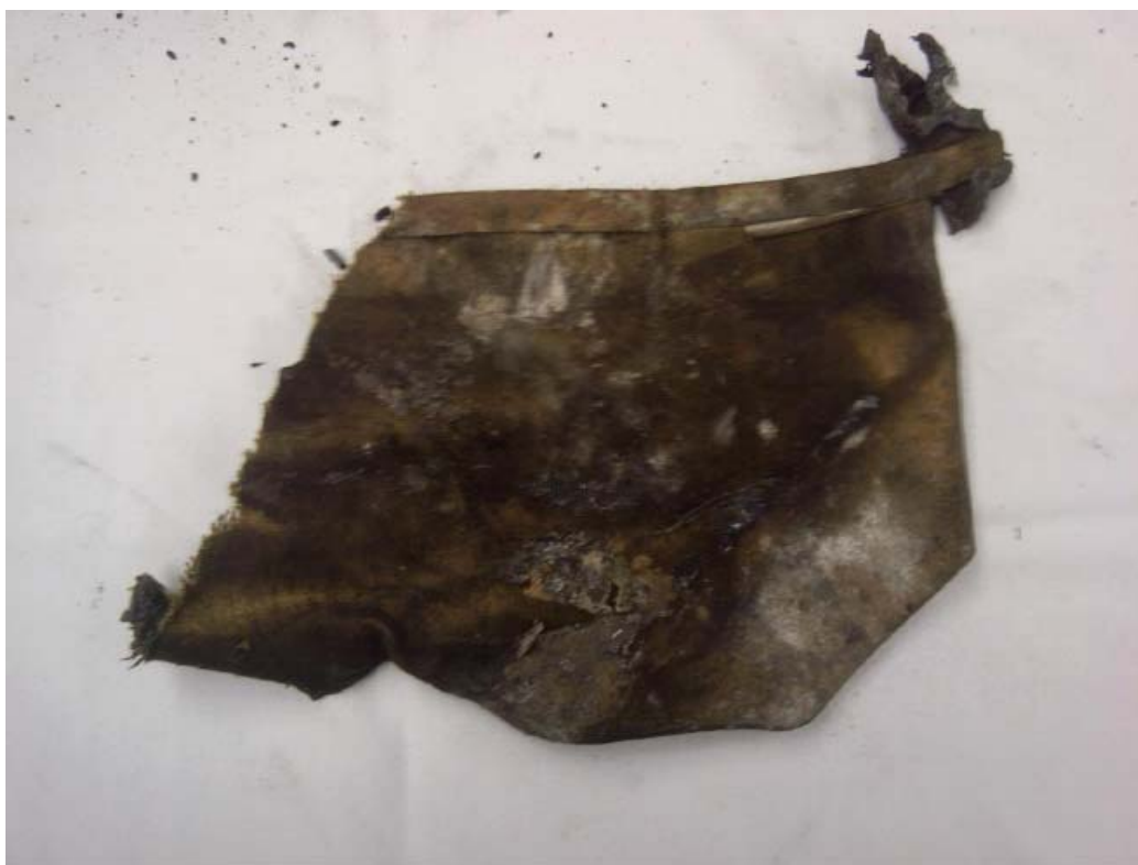
Portion of ear covers carbonized and burned away so Nomex exceeded 750 F.
