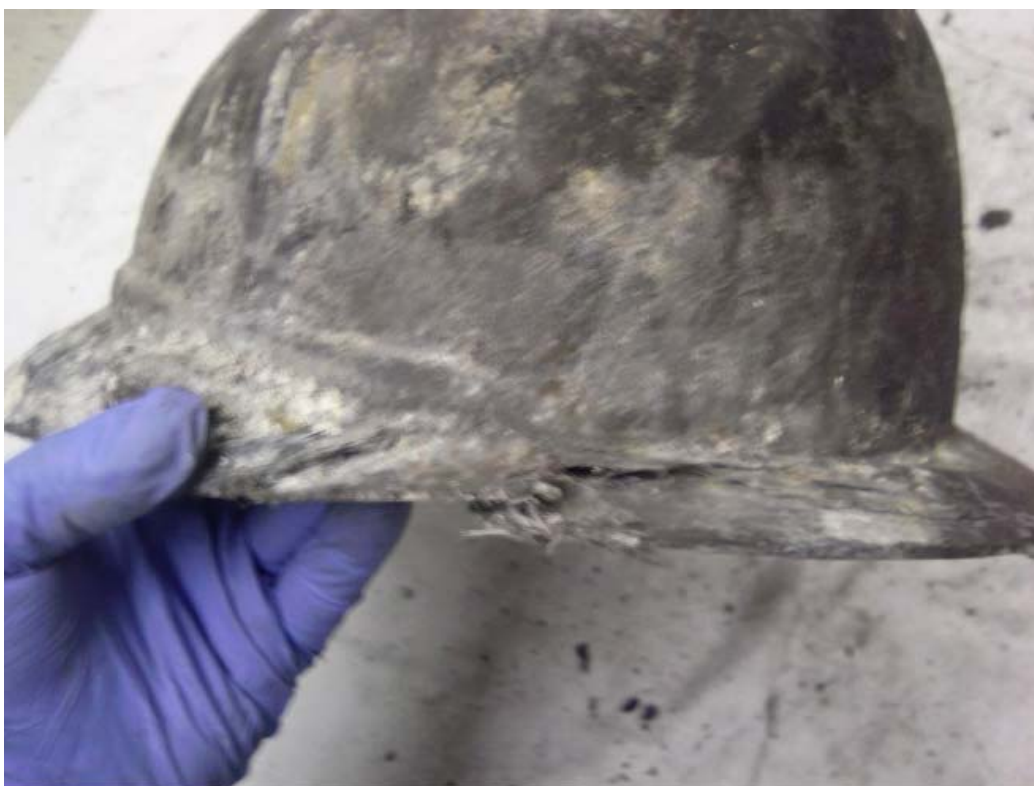
Helmet shell lay in direct contact with heat for so long portions of the shell had the resin burned away so had to reach way over 1000 F
