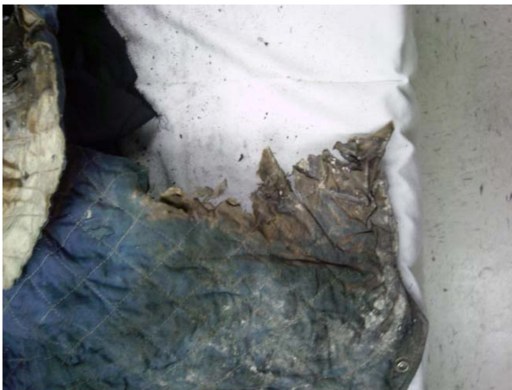
Liner totally carbonized / vaporized...at least 750 F and most likely over 1000 F
