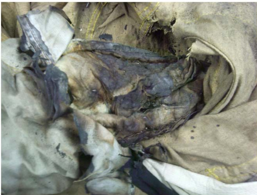
Large sections of the moisture barrier carbonized so reached at least 750 F in those areas. The Teflon underneath also carbonized as did these outward facing portions of the thermal liner and Dead Air Panels.
