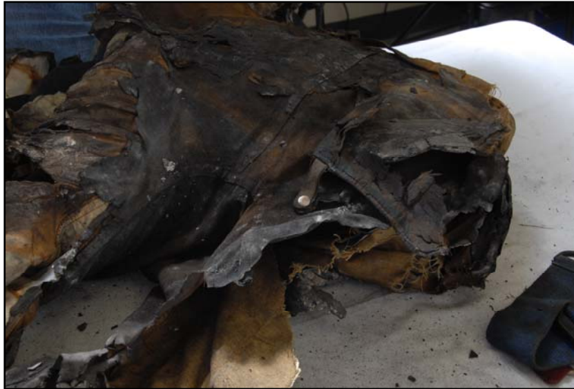
Figure 50: Seat and crotch area of Broxterman's trousers. Near complete degradation of rear and lower leg portions of the garment.
