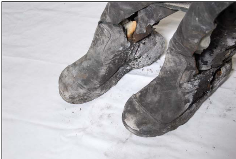
Figure 51: Thermally damaged leather footwear worn by Capt. Broxterman.
