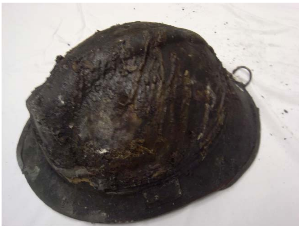
Yet again, Trim and ID markers on helmet carbonized. Massive amount of debris, molten carpet, etc. stuck to helmet.
