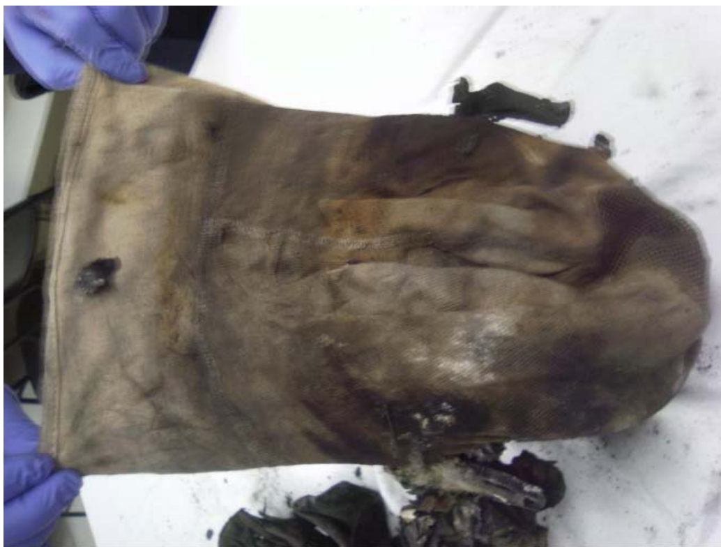
Pbi blend hood did char but remained intact. Note no charring in the 100% Pbi, ventilated area.
