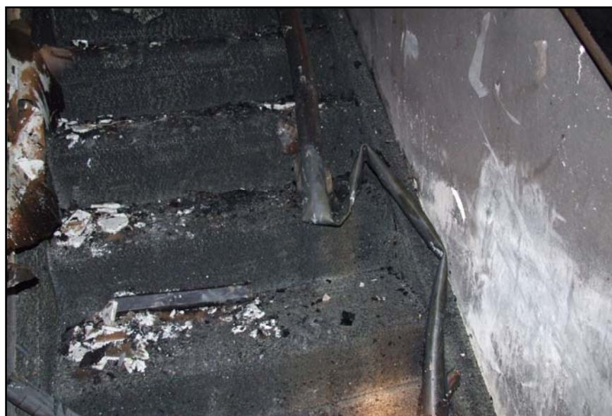
Figure 75: Burned away outer jacket of the attack hose line in the basement
