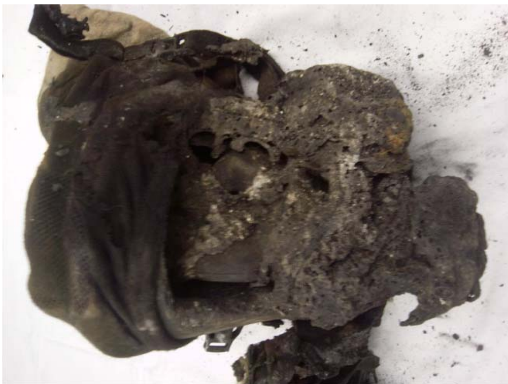
SCBA face piece, note carbonized portion of hood that reached in excess of 750 F
