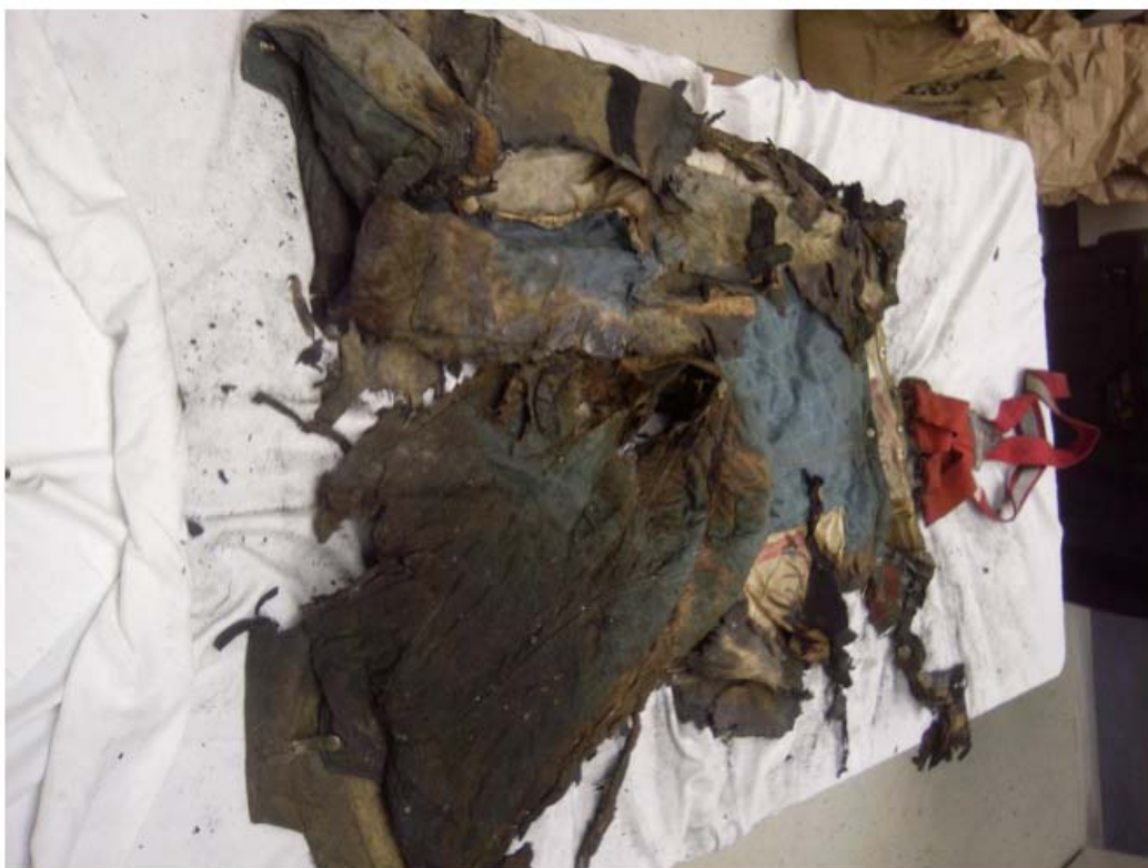
Literal thermal destruction of pant throughout most of the garment
