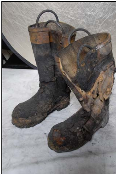
Figure 61: Thermally damaged rubber footwear worn by Ffr. Schira.
