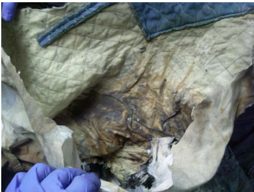
Charring shown here on outward facing side of thermal liner indicating it reached at least 750 F
