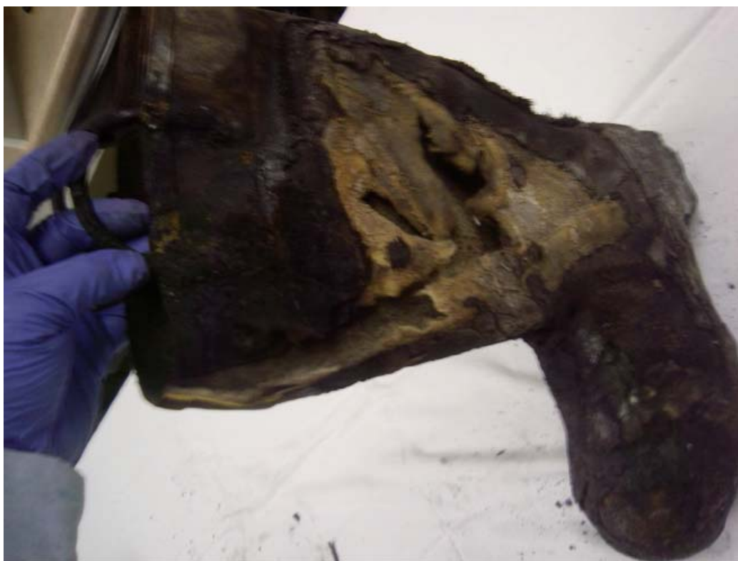
Portion of boots carbonized and the underlying Kevlar liner starting to char so reached around 900 F at the Kevlar layer
