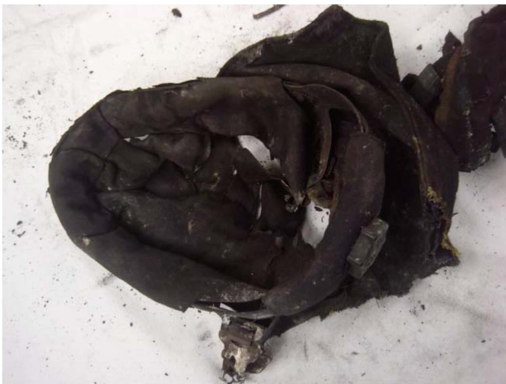
Helmet suspension intact but laying in fire for extended period finally separated it from the rest of helmet. Separation may have occurred when recovering FF Schira.
