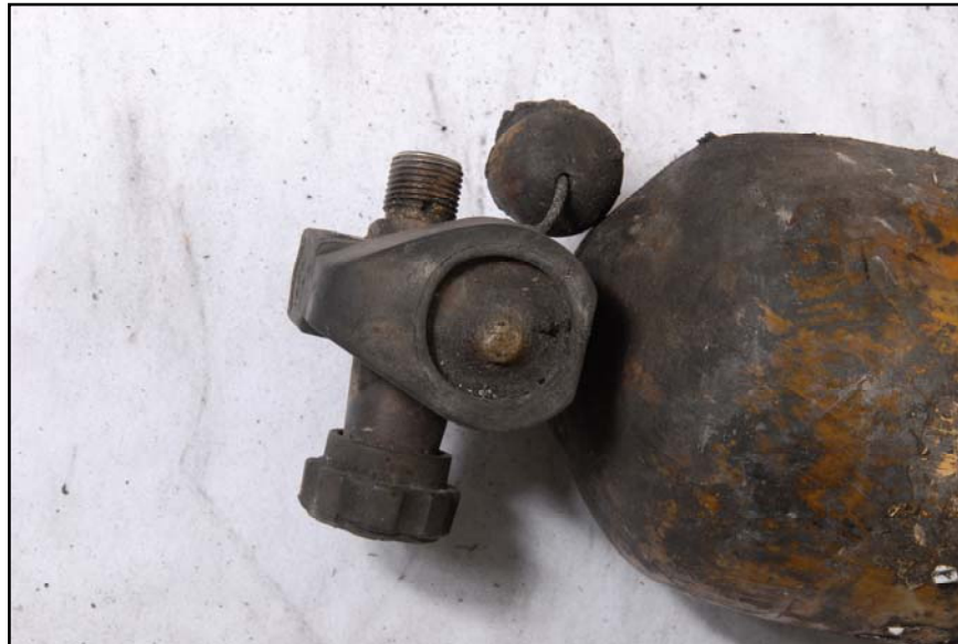
Figure 69: Ffr. Schira's breathing air cylinder pressure gauge thermal
