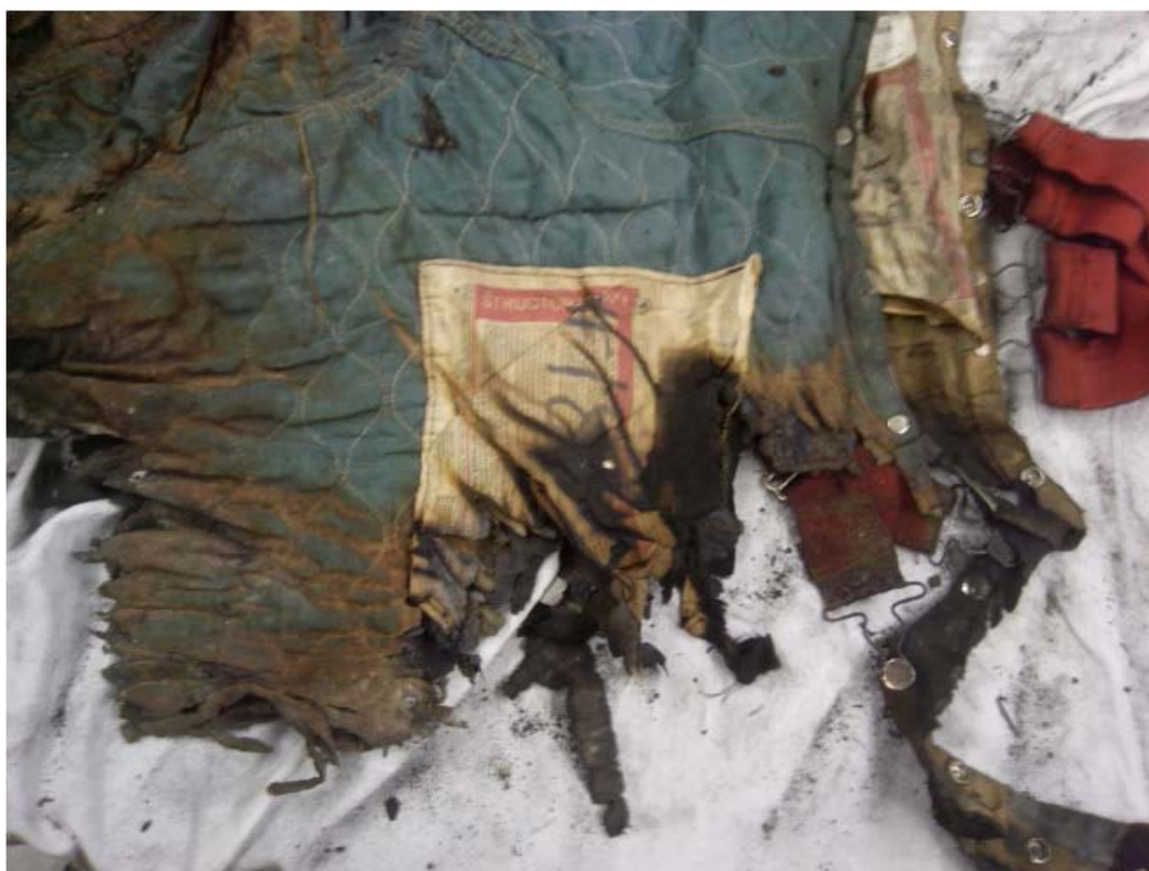
Left hip/buttocks area.....complete thermal destruction of Pbi shell requires 1300+ F, and underlying moisture barrier way over 750 F.
