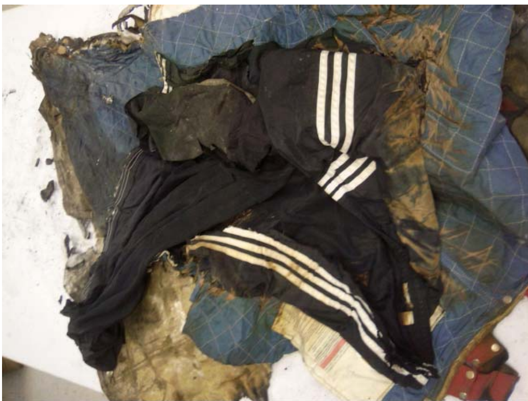
Work out pants being worn during the incident were melted and fused to the liner face cloth in areas.
