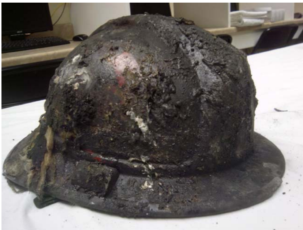
Again, Trim and ID markers on helmet carbonized. Massive amount of debris, molten carpet, etc. stuck to helmet.
