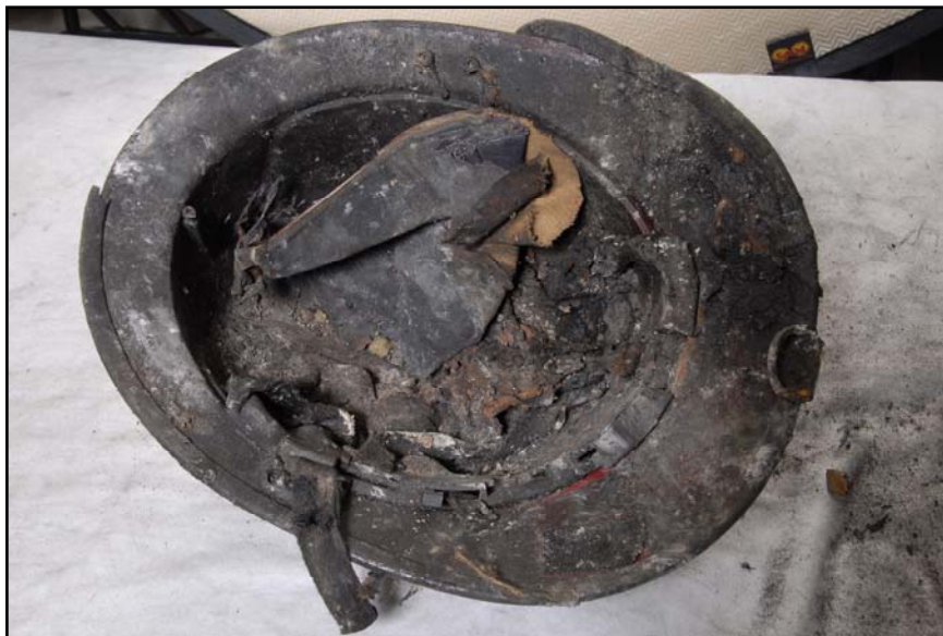
Figure 55: The heavily charred helmet outer shell interior along with remnants of the suspension system.
