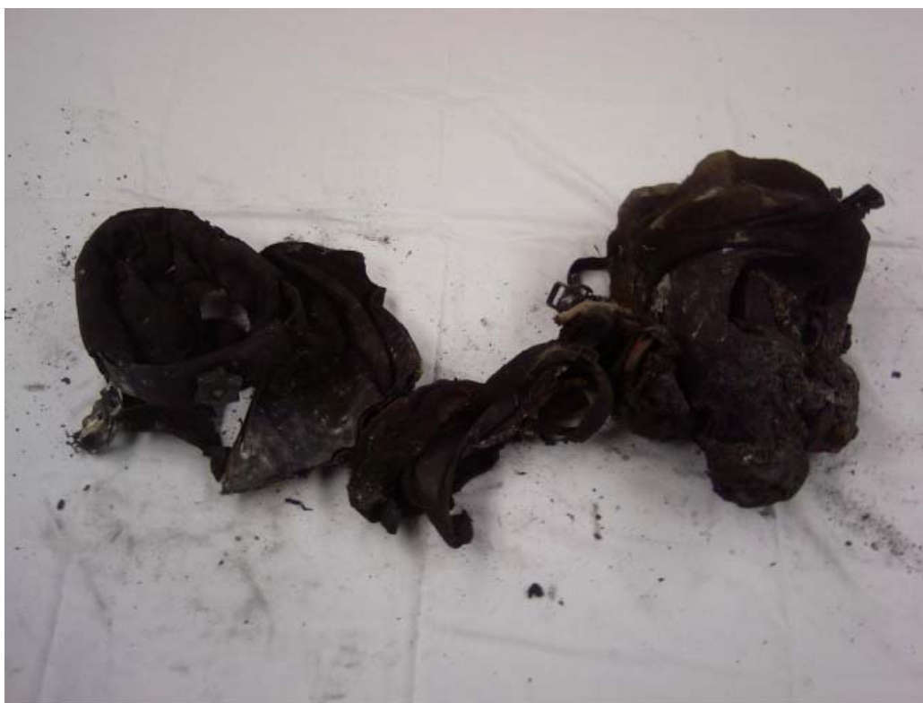
Helmet headband and SCBA face piece after laying in fire.
