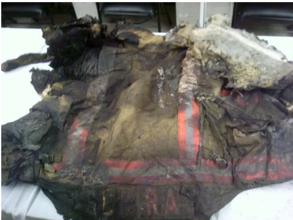
Rear of coat. Charred and carbonized Pbi reached at least 1300 F. Portions of trim were carbonized/vaporized.
