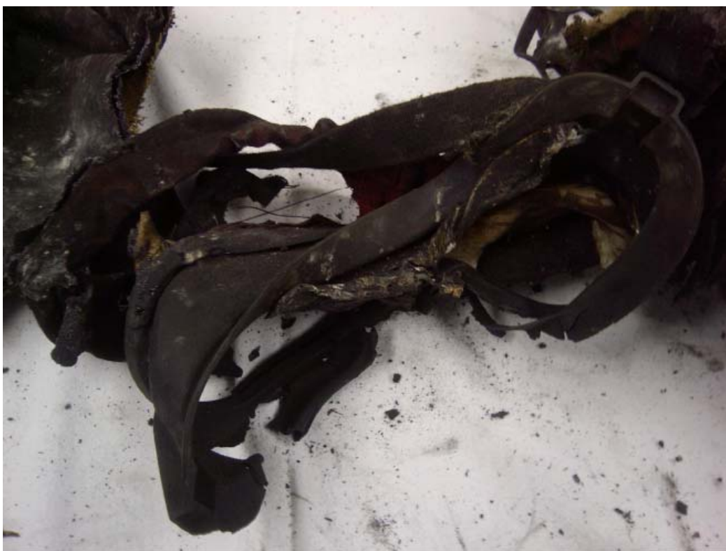
Lenses of goggles completely missing and presumed carbonized / vaporized
