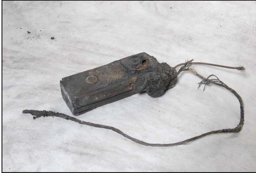
Figure 62: Remnants of Ffr. Schira's portable radio.
