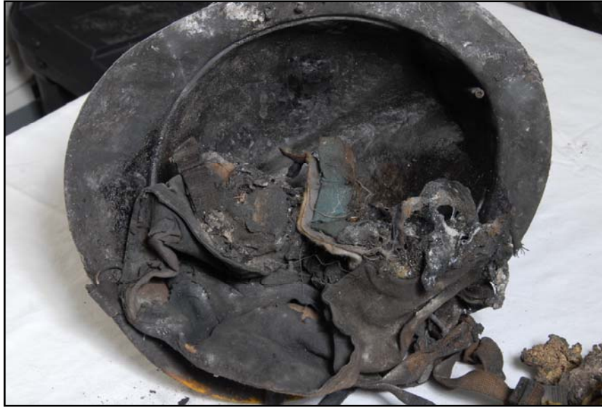
Figure 46: The heavily charred helmet outer shell interior along with remnants of the suspension system.
