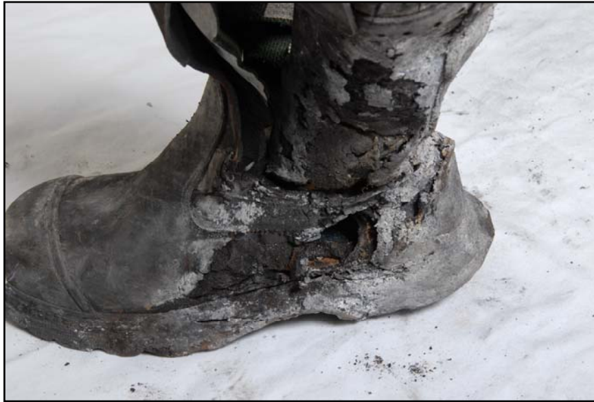
Figure 52: Significant full depth charring of the ankle and heel area.
