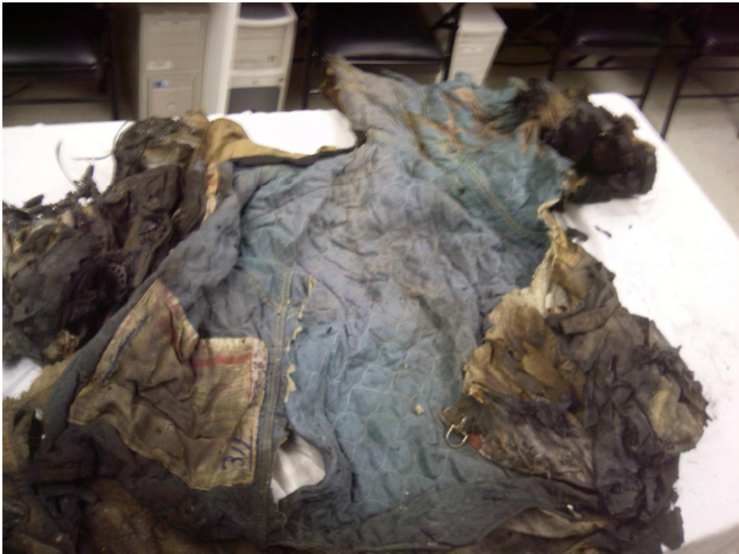
Massive thermal destruction penetrating all three layers of coat.
