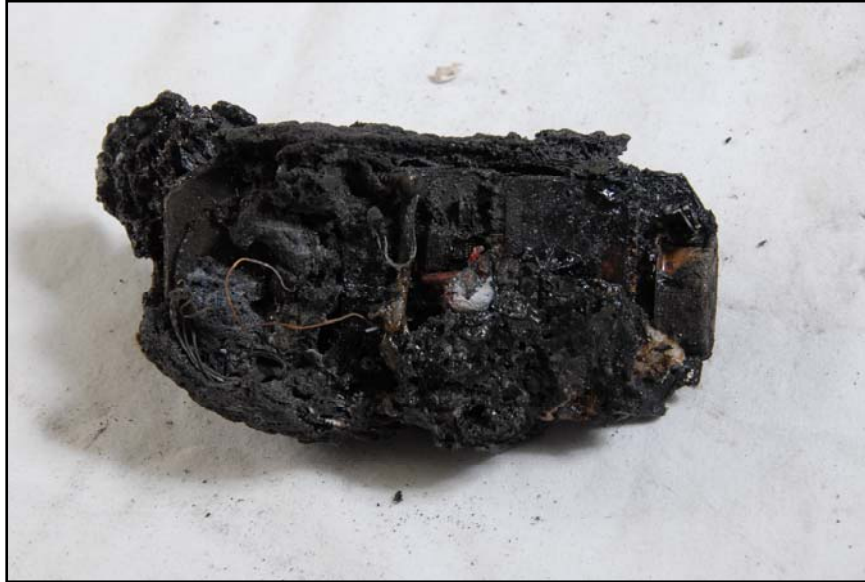
Figure 67: Captain Broxterman's thermally damaged ICM.
