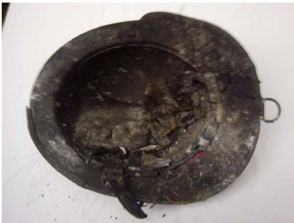
Helmet lay in the fire for so long it burned away the silicone edge beading and portions of the suspension mounting ring.
