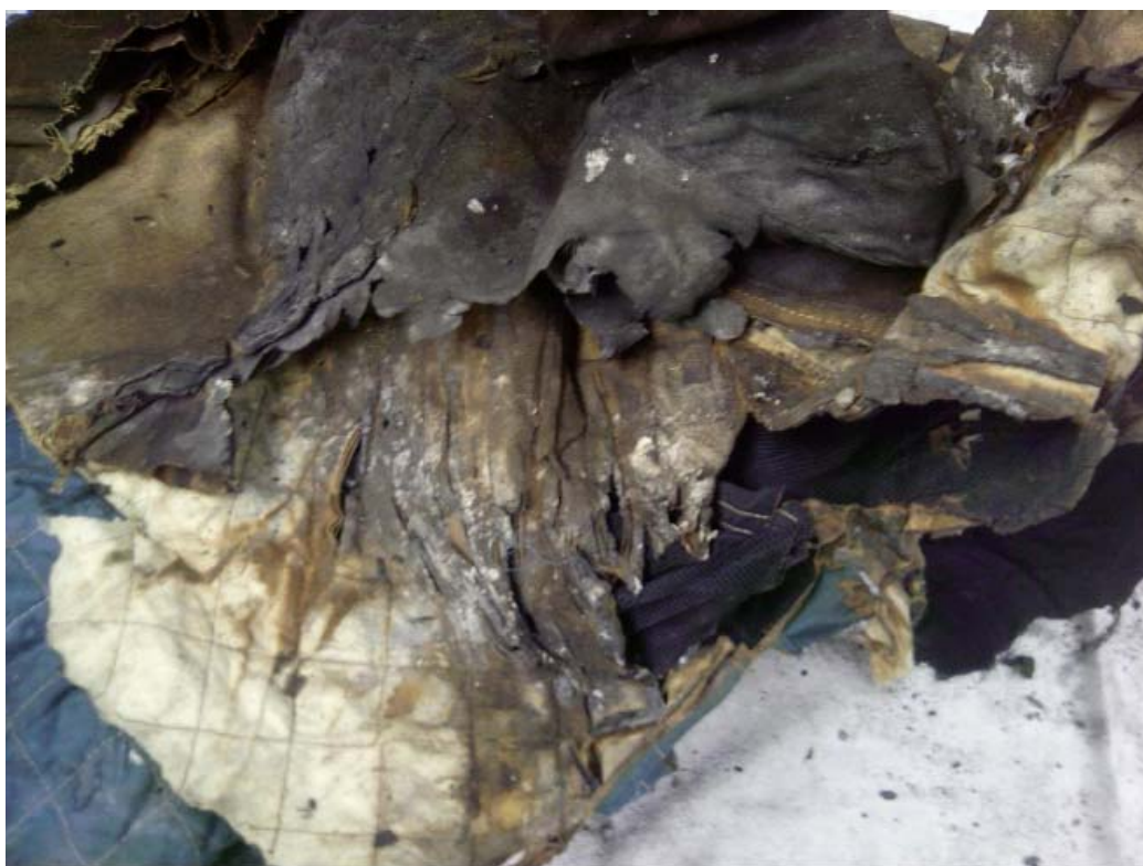
Shell 1330+ F. Moisture barrier way over 750 F. Parts of liner completed charred away, well in excess of 750 F and probably around 1000 F
