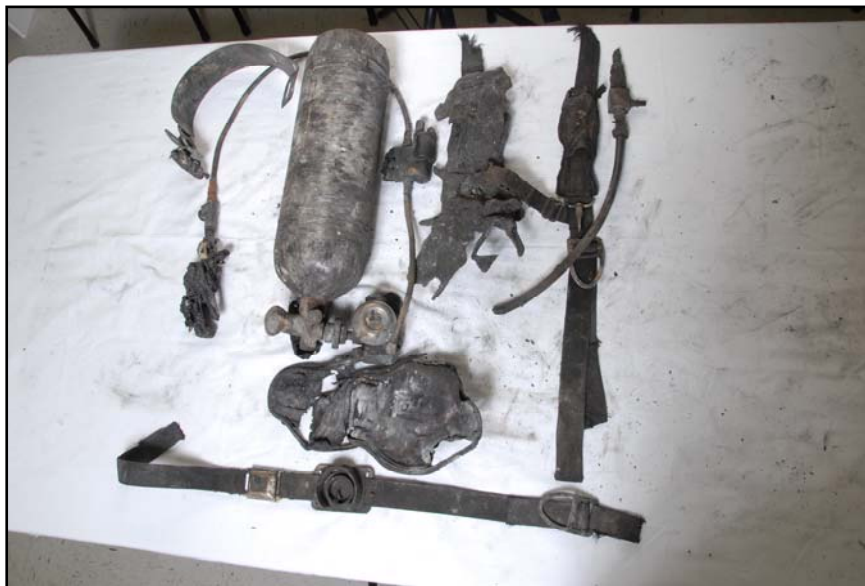
Figure 68: Thermally damaged remnants of Capt. Broxterman's SCBA assembly.
