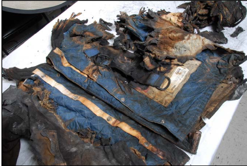
Figure 48: Rear of view of Broxterman's coat. Complete degradation back of coat. Note suspender hardware fused into lining material.
