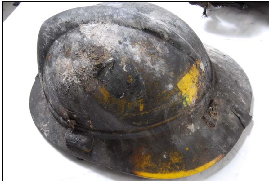
Figure 45: The heavily charred helmet outer shell worn by Capt. Broxterman.
