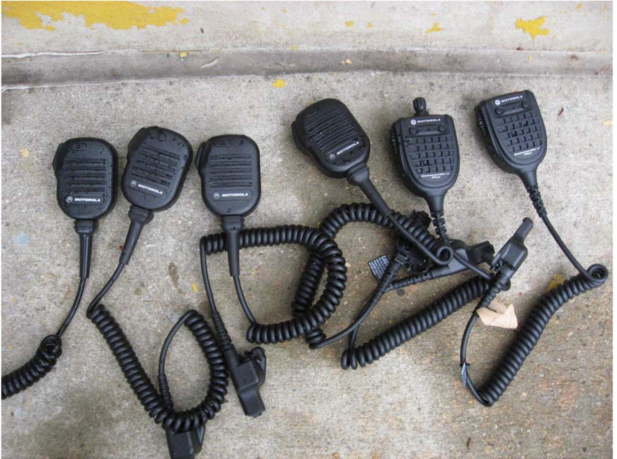
Motorola extended microphones used in testing model numbers NMN6193C, NMN6193BS03, NMN6191C, RMN5088A and RMN5066A
