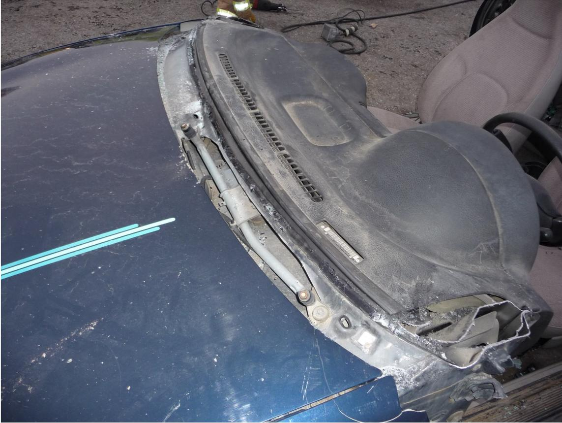
**If all goes as planned, the bottom of the windshield will dislodge from the Black polyurethane glue or mastic where it attaches at the top of the dash. You can relocate the roof and windshield out of the action circle as one.**
