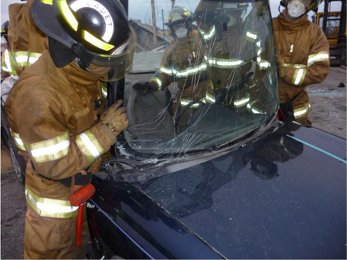
**At this point the rescuers will need to take most of the weight of the roof for a brief moment until it is past the 90 degree break-over point, and then continue to flip the roof over towards the hood.**
