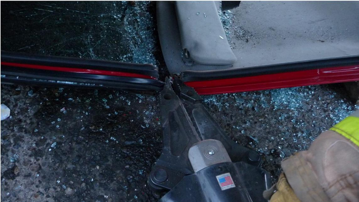
**When the spreader tips are expanded inside the cut, it will break away the roof and leave the complete windshield attached to the vehicle.**
