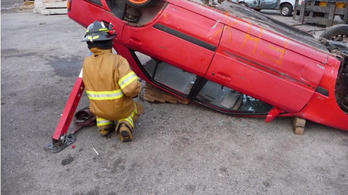
**When it is time to cut the A-pillars make the cut with hydraulic cutters at the top corners of the windshield as indicated.**
