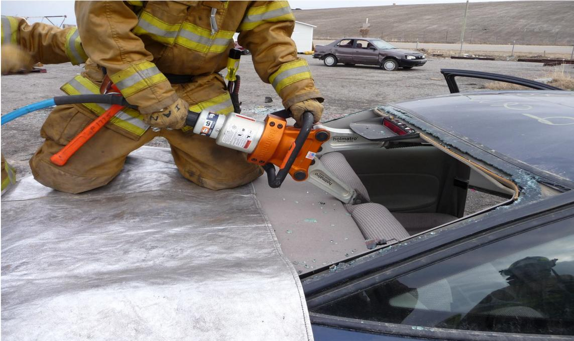
**Expand spreader arms to full extension, this will collapse the truck deck and create a “tenting” effect in the center of the roof producing a large enough hole for a rescuer to enter and a patient to be safely removed.**
