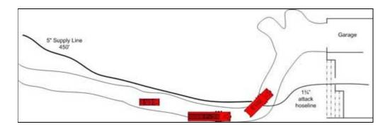
Diagram 3. Location of key fire apparatus and 1¾" attack hoseline from E102 into front door.
